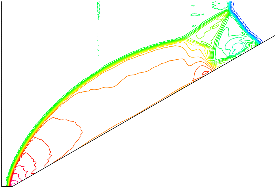
Figure 35. Computed density contours by the second DG method with the HWENO limiter for double Mach reflection of strong shock M_s = 10 .
